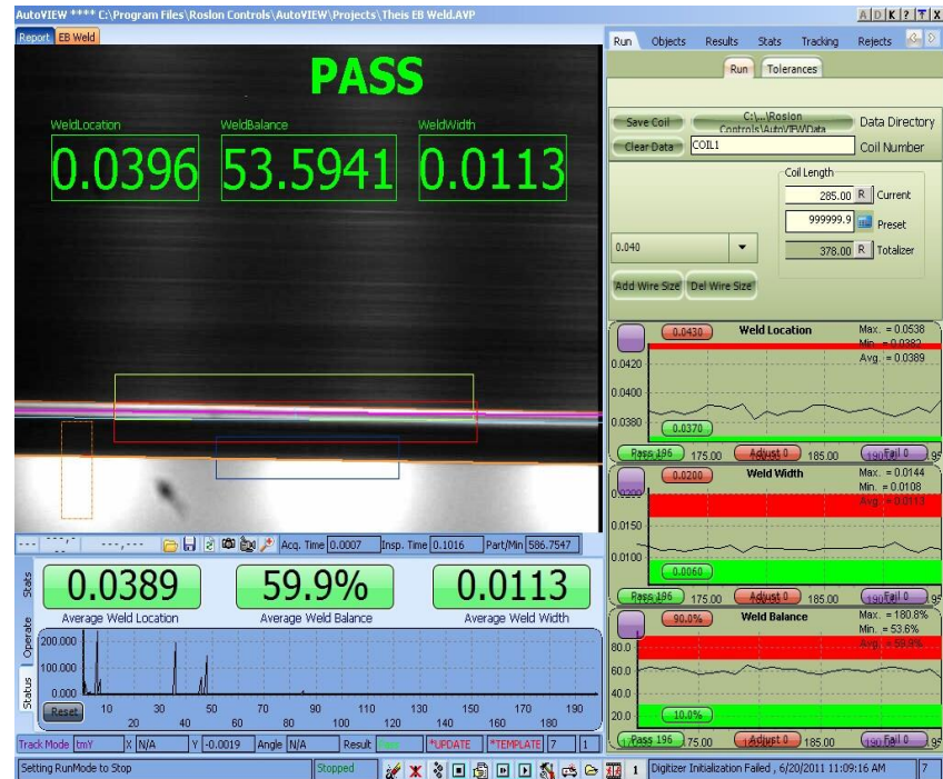
Continuous Weld Bimetal Strip Inspection Machine Vision Image Processing
